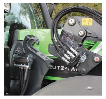
As the tractor drives into the frame, the front loader slides on to attachment until the locking pin touches the top of the slide rail.
