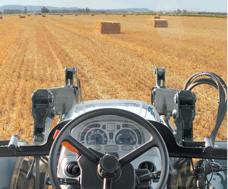
>> Because the loader is made from high strength steel, it can accommodate a particularly slim design. The view from the cab is optimal. K
