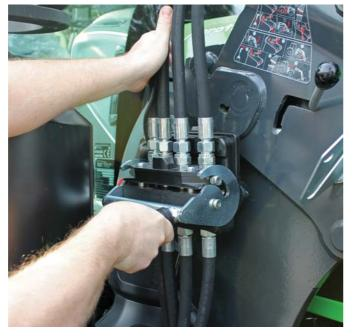
With the Hydro-Fix, all the hydraulic lines can be connected to the 2 tractor at the same time. The front loader is raised slightly in order to fix the locking pin in to arresting hook of the slide rail.
