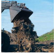
This is how it looks in practice: A full bucket is still a full bucket even as it is lifted, thanks to the rescooping function. The result: No trickle losses, high loading capacity. The system is as simple as it is ingenious. After lifting the loading bucket, the bucket can be tilted again by 24° while the loader is raised. Result: the load remains in the bucket.
