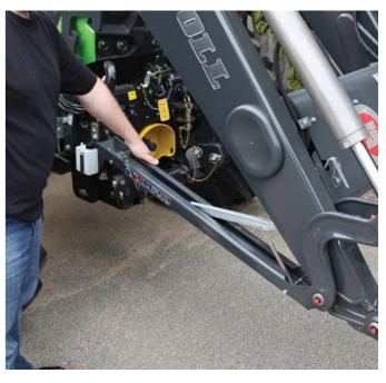
The parking supports can be folded in and out without tools. They automatically snap into the right position.
