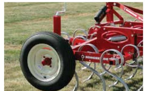
Crank Adjustment Gauge Wheel
