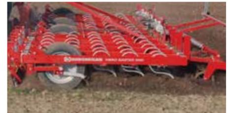
5 rows of tines in a symmetrical pattern ensuring a blockage-free passage of soil and residues.
