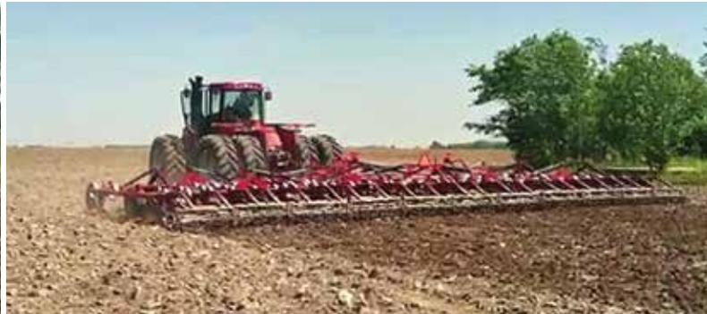
The Single Fold and Double Fold 8200 comes standard with heavy duty walking tandems on the mainframe and wings, front gauge wheels, single point hydraulic adjustment, drop leg jack, and a safety light kit.
