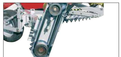
A V-belt pulley powers the stone rakes.
