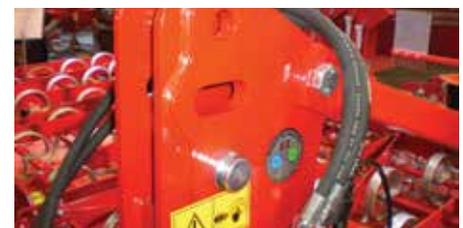
Slotted hole in the topmast helps the cultivator follow the soil surface in hilly conditions.
