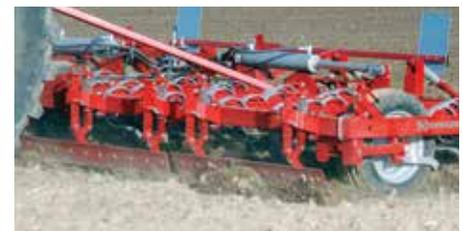
Levelboard with or without spikes for crushing and levelling the soil surface before entering the cultivation zone. Can be set to crushing or leveling mode.
