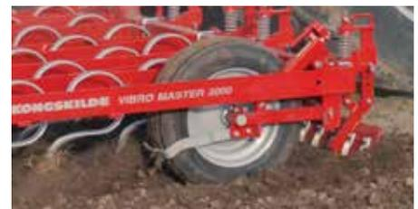
4 large rubber wheels running in front of the tines on firm soil for even depth control.
