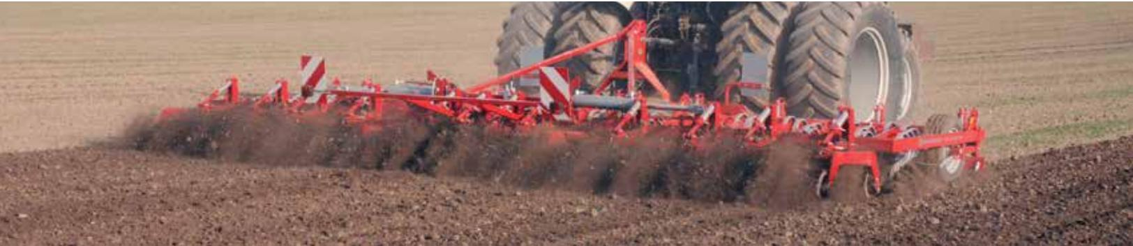
Kongsilde Vibro Master 3000 is a fully-mounted seedbed cultivator equipped with vibrating tines in working widths from 21' to 27', for tractors up to 250 hp.
