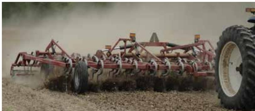
Kongskilde's Model 8200 cultivator series has 6 rows of shanks which allows for unmatched residue clearance with tines in 4" (10 cm) or 6" (15 cm) centers. The framework is 4" (10 cm) x 4" (10 cm) x 1.4" (0.635 cm) wall thickness. The framework is extruded through all frame members for added strength. The frame is 162" (4.115 m) from the front tine bar to the rear tine bar.
