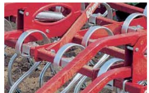
Oval Beam-Truss frame design for added strength.
