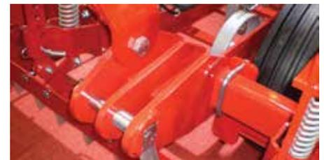
Lower linkage Cat. 2 and 3. Linkage pins are protected from rotation and wearing.
