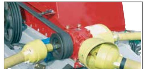
The rotor is powered by a reversing gearbox and a straight V-belt pulley.
