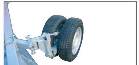
Adjustable double wheels control the depth of the SB 5200 stone rakes.
