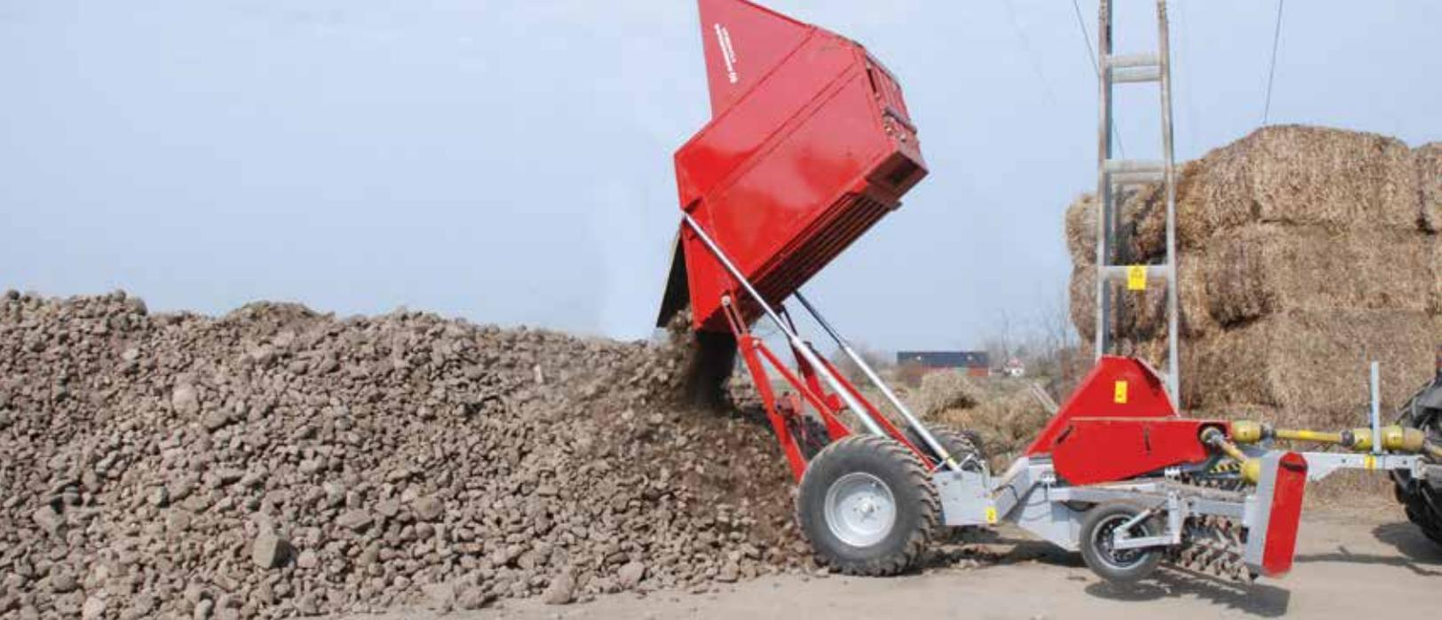
The hopper design on the Stonebear is with a 1.8 cu. m capacity. The hopper has small holes in front to indicate the level and inform the operator for emptying.
