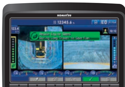
Eco-gauge, Eco guidance and fuel consumption gauge
