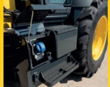
*AdBlue®, fuel and hydraulic oil tank are easily accessible on the machine side and refilled by ground level, ensuring a fatigue less operation*
