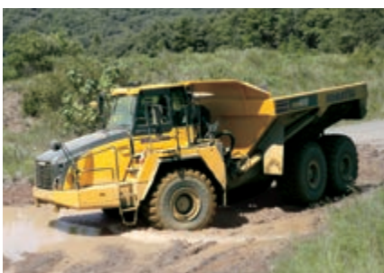
Komatsu Traction Control System (KTCS): maximum machine performance on soft and slippery ground
