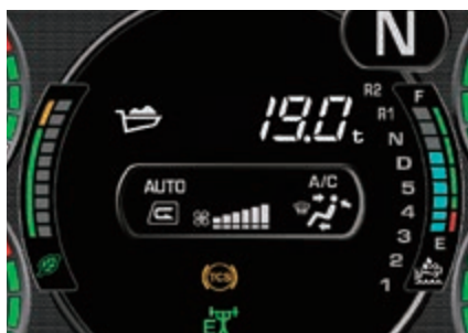
Payload meter displays the loaded weight
