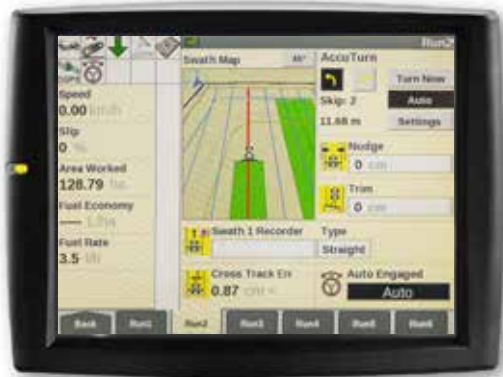
Automated turning process with AFS AccuTurn Pro
