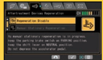
Aftertreatment device regeneration screen for the KDPF
