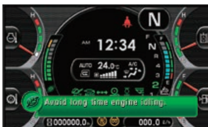
Eco-gauge and an Eco guidance with active recommendations help maximising fuel savings
