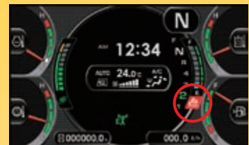
AdBlue® level gauge and refill guidance
