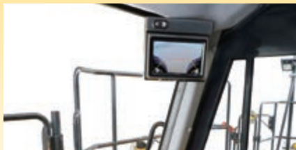
The separate rear-view monitor can be always on (only when reversing)
