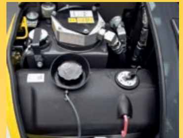
Convenient and save fuel and oil refilling under the front bonnet
