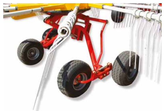
500 mm ground clearance at headland turns
