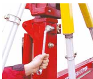
The width is adjusted mechanically at the rotor arms.
