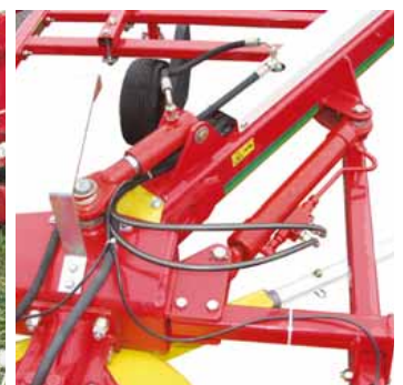
Hydraulic working width adjustment
